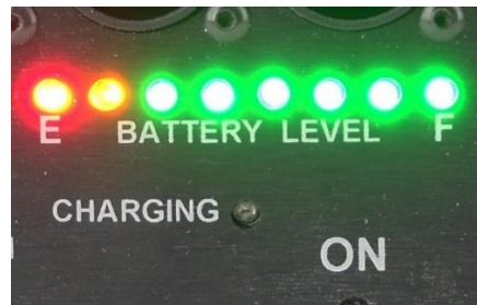
Battery “Fuel Gauge” indicating a fully charged battery
