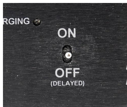
Power “ON” and “OFF” Switch. Note, to turn off unit you must hold switch in the “OFF” position for 4-5 seconds
