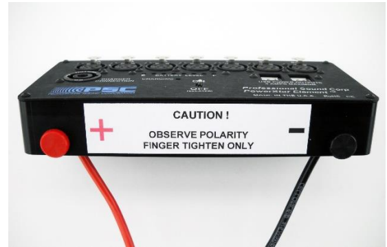
Cable attached to Power Star Element
